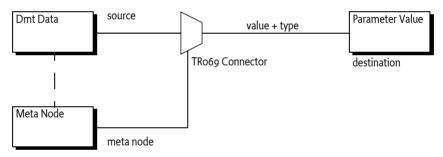
The different conversions possible for the Dmt Data to the TR-069 Parameter value are shown in Table 131.6. This table shows vertically the Dmt Admin formats and horizontally the TR-106 types defined in Table 131.5. Each row has a default conversion type, indicated with a bold entry. For example, the default conversion of a FORMAT BOOLEAN to the boolean type is the default conversion.
