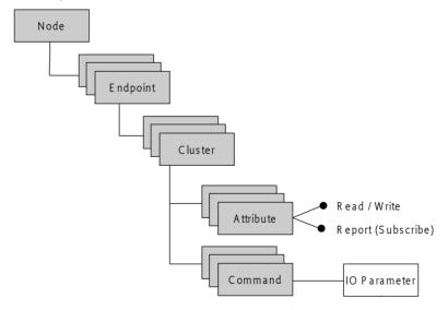
All interfaces corresponding to the ZigBee Cluster Library model (see Figure 149.5 on page 1021) must be implemented in order to discover and control asynchronously ZigBee devices. Classes related to the description of these entities named with suffix Description may optionally be implemented. This rule follows the fact that ZigBee device descriptions are not downloadable on the device itself and are often given to developers in an out-of-band manner.
