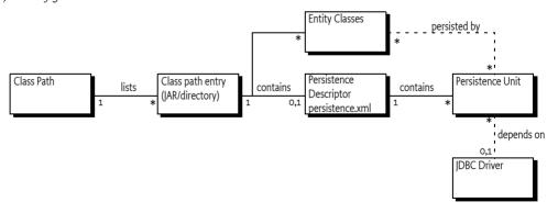
JPA recognizes the concept of a *persistence root*. The persistence root is the root of the JAR (or directory) on the class path that contains the META-INF/persistence.xml resource.
