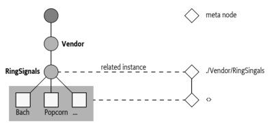
A URI is generally associated with the same Meta Node. The getMetaNode(String) should return the same meta node for the same URI except in the case of *Scaffold Nodes* on page 385. As the ownership of scaffold nodes can change from the Dmt Admin service to the Parent Plugin service, or from a Parent Plugin to a Child Plugin, the Meta Node can change as well.
