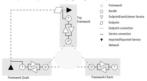
The previous description is just one of the possible usages of the Endpoint Event Listener. For example, the discovery bundles could communicate the scopes to their peers. These peers could then register an Endpoint Event Listener per peer, minimizing the network traffic because Endpoint Descriptions do not have to be broadcast to all peers.
