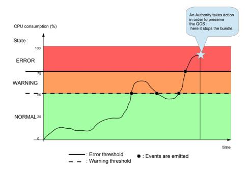
In this example, only the upper threshold is set. The upper warning threshold is set to 50%, the error one is set to 75%. CPU consumption fluctuates between 0 and 50%, the usage is in the NOR-MAL state. Then it increases and reaches 50%. The usage then goes from the NORMAL state to the WARNING state and the Resource Listener holding the threshold receives a WARNING Resource Event.
