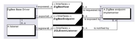
To control ZigBee devices, a bundle should track ZigBeeEndpoint services in the OSGi service registry and control them appropriately. OSGi applications can browse the clusters (ZCLCluster objects) that are discovered on every registered ZigBeeEndpoint and attributes (ZCLAttribute objects) that are discovered on every ZCLCluster. They can invoke commands on these clusters and get the current value of attributes.
