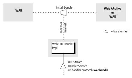
When the Web Container bundle is installed it must provide the webbundle: scheme to the URL class. The Web URL Handler has two primary responsibilities:
