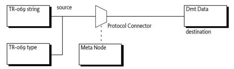
The destination type is obtained from the corresponding Meta Node. If multiple formats are specified in the result of the <code>getFormat()</code> method then the most applicable type must be used. The following table lists the applicability for each TR-106 data type.
