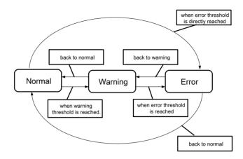
A threshold state depends on the current consumption of resource and the type of threshold (upper or lower threshold).
