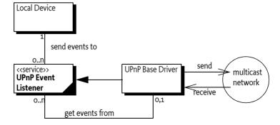
If a service is registered with a property named upnp.filter with the value of an instance of an Filter object, the listener is only notified for matching events (This is a Filter object and not a String object because it allows the InvalidSyntaxException to be thrown in the client and not the UPnP driver bundle).
