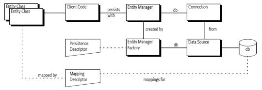
The JPA specifications define a number of concepts that are defined in this section for the purpose of this OSGi specification. However, the full syntax and semantics are defined in the JPA specifications.
