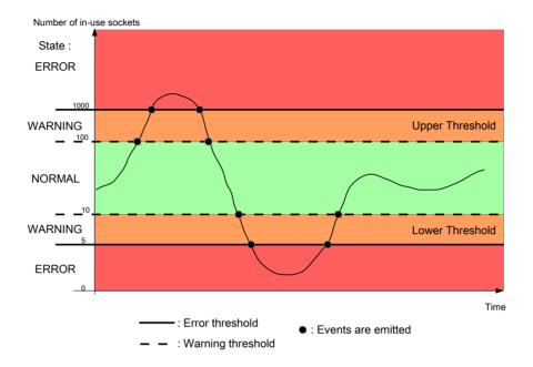
In our example, the lower warning threshold and the lower error threshold of the Resource Listener are respectively set to 10 and 5. When the number of in-use sockets decreases under 10, the usage goes from the NORMAL state to the WARNING state and the Resource Listener receives a WARNING event. If the number of in-use state sockets decreases again and goes down to 5, the usage goes from the WARNING state to the ERROR state and the Resource Listener receives a ERROR Resource Event.
