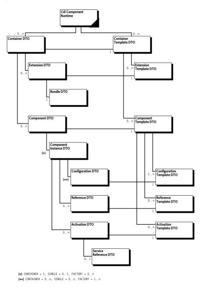
The ContainerDTO specifies a changeCount field of type long. Whenever the DTOs bellow the ContainerDTO change, CCR will increment the ContainerDTO's changeCount. Whenever any ContainerDTO changes, CCR will update the service.changecount service property of the CDIComponentRuntime service. CCR may use a single update to the service.changecount property to reflect updates in multiple ContainerDTOs. See org.osgi.framework.Constants.SERVICE\_CHANGECOUNT in OSGi Core Release 8.
