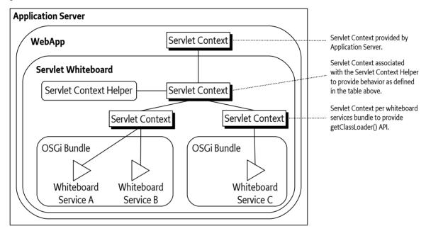
Where Table 140.2 on page 789 states *Backed by the Servlet Container* and the Servlet Whiteboard implementation is deployed in bridged mode, the API call can be forwarded to the top-level Servlet Context. If the Servlet Whiteboard implementation is not deployed in bridged mode, it must provide another means to handle these APIs.
