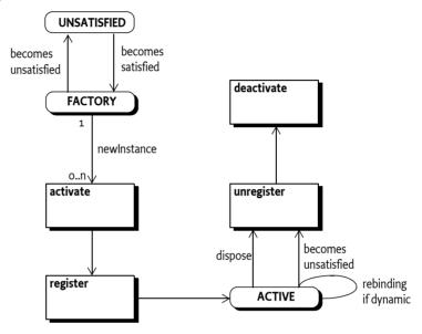
A Component Factory service has a single method: newInstance(Dictionary). This method must create, satisfy and activate a new component configuration and register its component instance as a service if the component description specifies a service. It must then return a ComponentInstance object. This ComponentInstance object can be used to get the component instance with the getInstance() method.
