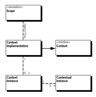
The *component scope* is a [9] *Pseudo-scope* identified by the @ComponentScoped annotation. The *component scope* allows component instances to use component beans to create or destroy contextual instances when dependencies are satisfied or unsatisfied without interfering with the life cycle of other component instances (including the container component).
