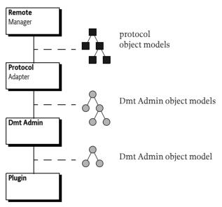
If an object implements a standardized data model it must be visible through its *native* Protocol Adapter, that is the Protocol Adapter that belongs to the object model's standard. For example, an ExecutionUnit node defined in UPnP Device Management could be implemented as a bundle, exposed through a Data Plugin for the Dmt Admin service, and then translated by its native UPnP Protocol Adapter.
