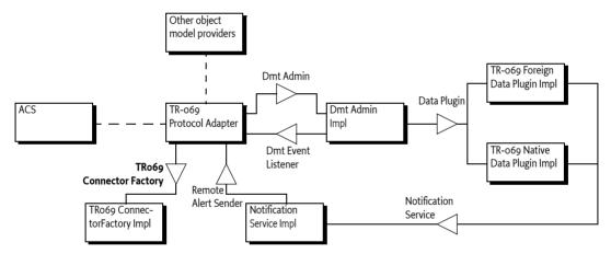
The Protocol Adapter can be implemented as an OSGi Bundle or it can be implemented in native code in the device. Both architectures are viable. For certain aspects like the TR-157a3 Software Modules a certain amount of native code will be required to manage the OSGi Framework as an Execution Environment.
