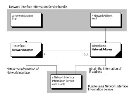
The NetworkAdapter service provides the network interface information for a logical interface. NetworkAddress service provides the IP address information for an IP address. A NetworkAddress service is associated with a NetworkAdapter service.
