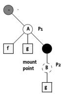
If the child node names are requested for the ./A node then the plugin P1 is asked for the child node names and must return the names [f,g]. However, if plugin P2 is mapped then the Dmt Admin service must add the scaffold node name that makes this plugin reachable from that level, the returned set must therefore be [f, g, X].
