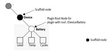
A scaffold node is always an interior node and has limited functionality, it must have a type of DDF\_SCAFFOLD. It has no value, it is impossible to add or delete nodes to it, and the methods that are allowed for a scaffold node are specified in the following table.
