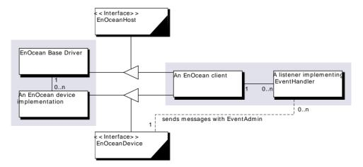
Client bundles may also expose framework-internal (local) EnOceanDevice instances, registered within the framework, see Figure 139.3 on page 764. The Base Driver then should emulate those
