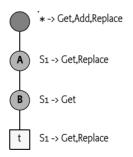
Figure 117.20 demonstrates the effect of this rule with an example. Server S1 can change the ACL properties of all interior nodes. A more detailed analysis:
