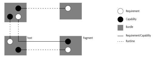
The core does not specify a namespace for services. However, services can also be modeled with requirements capabilities. The registrar is the provider and the service properties are the capability. The getter is the requirer, its filter is the requirement. This specification therefore also defines a namespaces for services:
