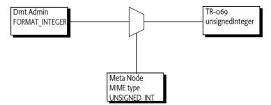
Since a Meta Node can contain multiple MIME types, there is no restrictions on the number of Protocol Adapters; a Plugin can specify the MIME types of multiple Protocol Adapters.
