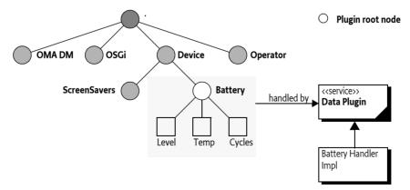
Plugins are OSGi services. The Dmt Admin service must dynamically map and unmap the plugins, acting as node handler, as they are registered and unregistered. Service properties are used to specify the sub-tree that the plugin can manage as well as mount points that it provides to *Child Plugins*; plugins that manage part of the Plugin's sub-tree.
